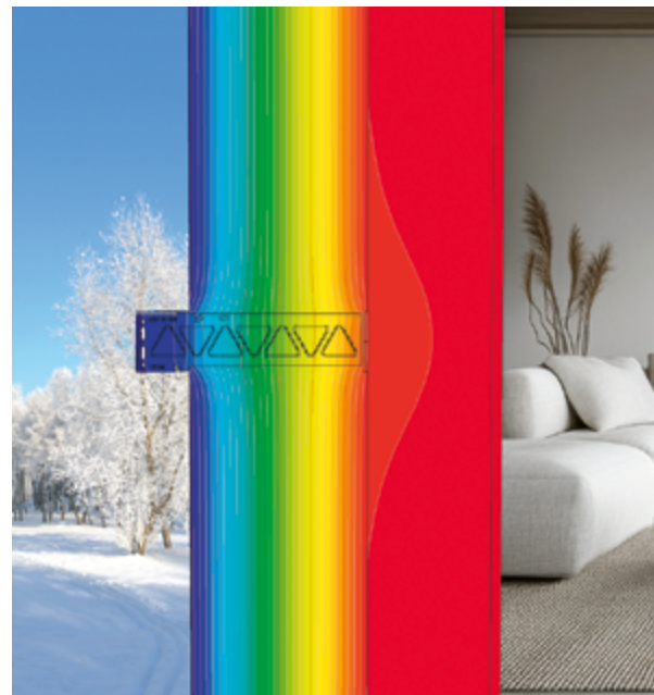
Image 2 Minimal thermal bridge with CROSSFIX®
